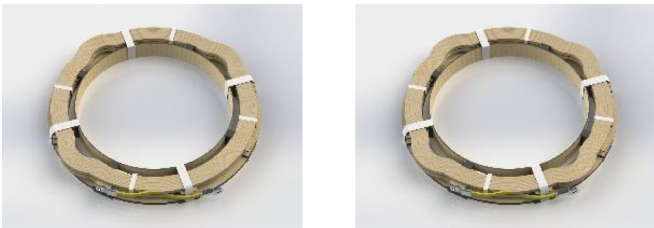
Fig. 5. Sketch of winding radial deformation.
