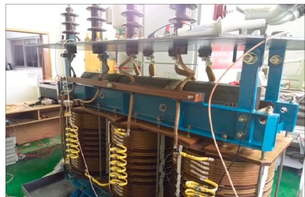
Fig. 12. Tested model transformer with its tank uncovered. (a) Internal configuration of model transformer. (b) An image of model transformer.
